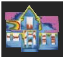
Before siding insulation. Energy transfers through the studs and siding.
